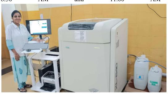
**Radiology Department** A fully Networked Computer Radiography System with Minipacs has been installed for film less functioning.
